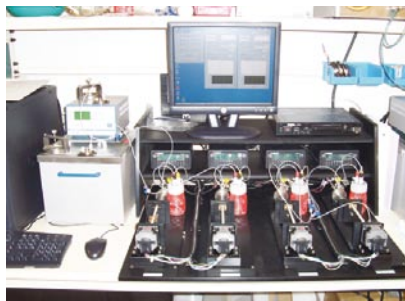
Figure 3. Reservoir pressure-volume test system uses motor actuated syringes to vary the pressure
